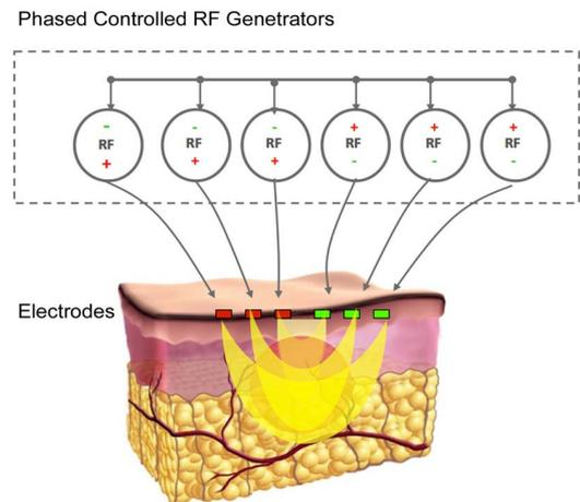
**Figure 1.** Configuration of six phase controlled RF sources as implemented in the Endymed Pro multisource technology. Multisource RF technology is based on the fact that flow of energy on the surface is minimal, while all energy is directed to the depth of the tissue. This is achieved by repulsion between electrical field of the same polarity on each side of the handpiece.
